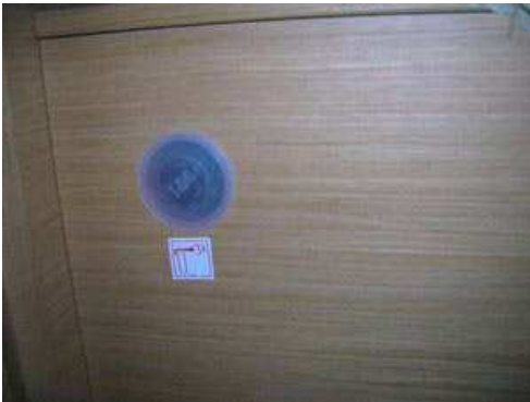
Extinguisher hole located under the companionway step - (Reference 2) A diagram enables it to be found easily
