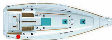
Drainage through suction outlet - Starboard catwalk
