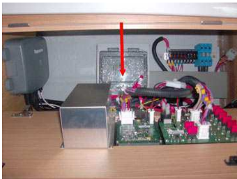
Decompounded switch 40A - Back of electrical panel
