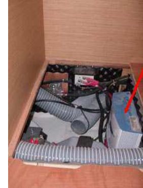
Battery charger - 40A Starboard aft cabin
