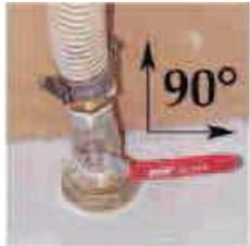
Thru-hull fitting closed
