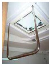
The ladder rung fitted to the ceiling enables evacuation through the forward deck hatch once removed from its storage.
