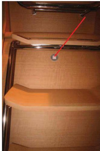
Extinguisher hole located under the companionway step
